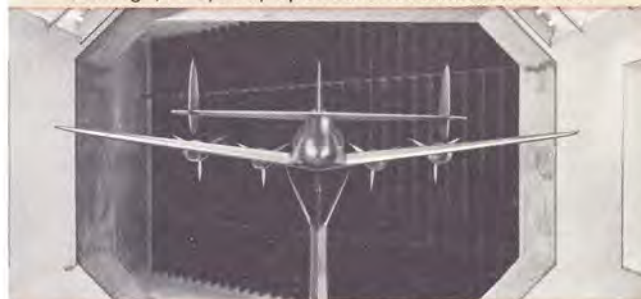
Nine-foot powered Constellation scale model was tested in throat of 300-mph wind tunnel.
