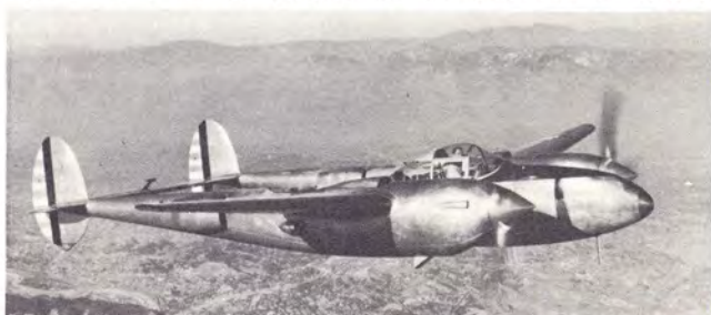
YP-38, nicknamed "Yippee," succeeded lighter XP-38, was armed with 37 mm. cannon, four .50 caliber guns.
