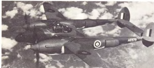
Dubbed "Lightning" by British, Model 322 P-38 lacked usual turbo-superchargers. British later added them.
