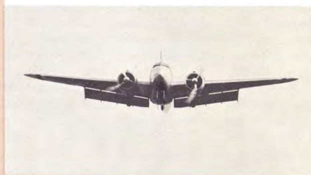
Lowered flaps shortened takeoff run. Development won 1937 Sperry award for Engineer C. L. Johnson.
