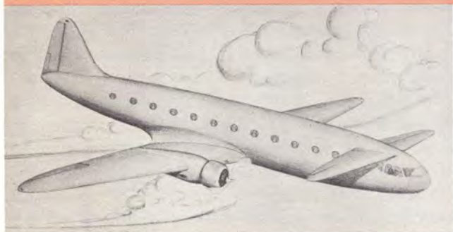
Canard transport designed in late 1930s had horizontal control in nose, aroused great interest but no orders.
