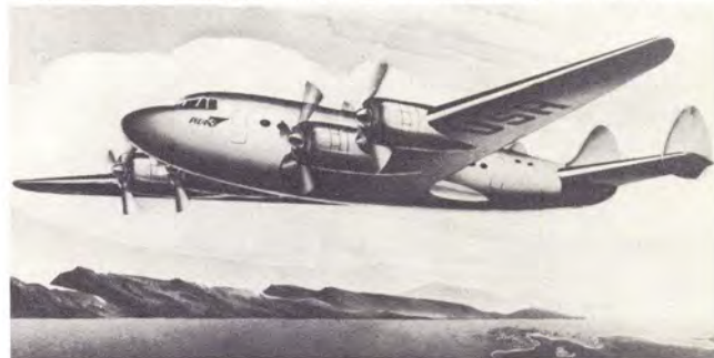
Pan American Airways wanted Excalibur larger and faster to carry 34 passengers plus crew at 300 mph top speed.
