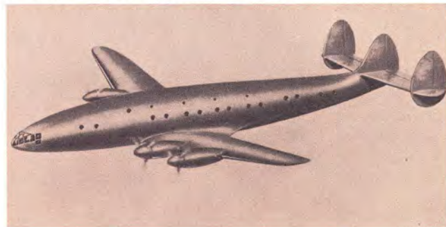
As originally conceived in 1939, Constellation showed faired nose, reverse flow cowling for its Wright 3350s.
