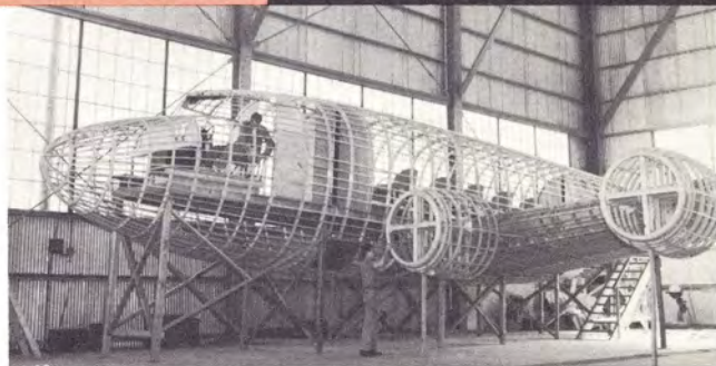
Excalibur design built as mockup in 1938-39 was a four engine airliner larger than Lodestar, smaller than DC-4.
