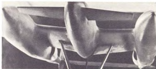
Control surfaces were located ahead of wing in canard version of P-38, abandoned after wind tunnel testing.
