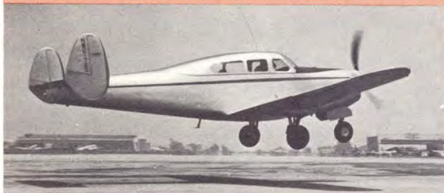
Starliner, shown taking off at Union Air Terminal, featured tricycle landing gear, "Unitwin" engine.
