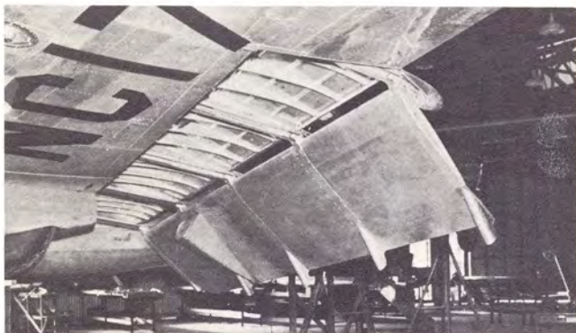
Lockheed-Fowler flap slid backward out of wing to increase wing surface during takeoff and landing.
