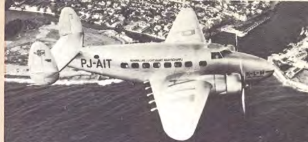
KLM Super Electra flying over Rotterdam showed guide rails trailing behind wing for Lockheed-Fowler flaps.
