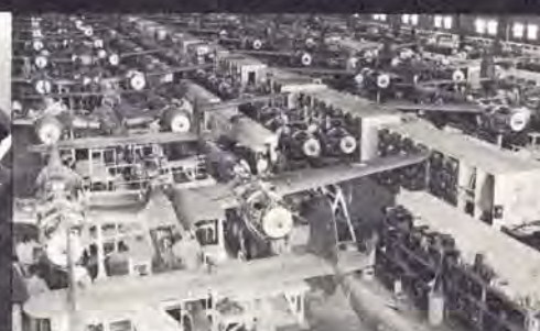
Moving conveyor line mechanized P-38 assembly, boosted output 72 per cent.
