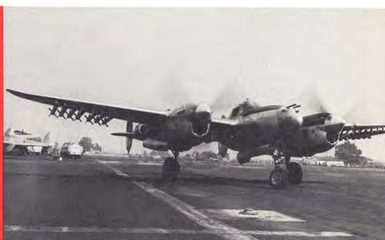
Fourteen rockets slung under Lightning's wing provided firepower equal to Navy cruiser's six-inch broadside.
