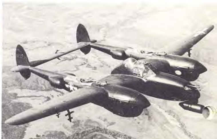
Night fighter P-38 provided cockpit for radar operator, mounted small pod below nose to house radar equipment.
