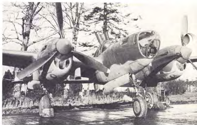
"Droopsnoot" version had elongated nose for bombardier, Norden bombsight, bombing and navigating instruments.
