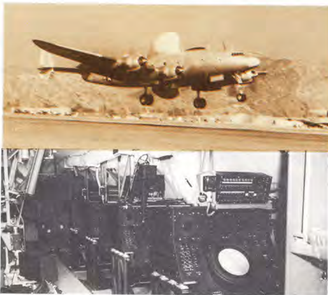
First in long series of aerial pickets that help guard America against enemy attacks was PO-1W Connie (upper photo) that had first flight in June 1949. The planes bulge with electronic scanning devices (below).
